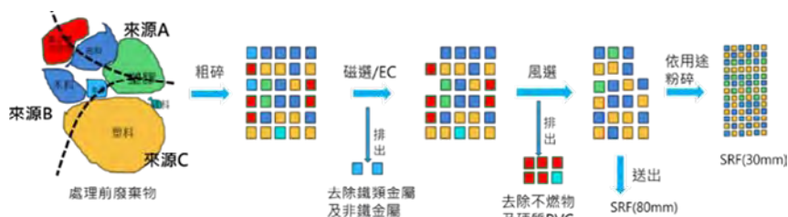
▲ Schematic diagram of the SRF process
