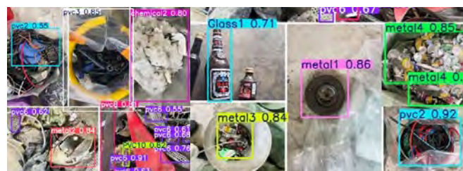
▲ dataset simulating waste on the conveyor belt by the team
